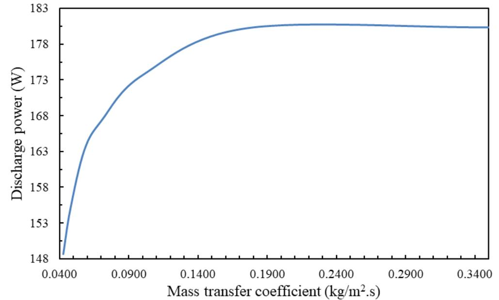
The performance is limited by mass transfer resistance of the solution film
