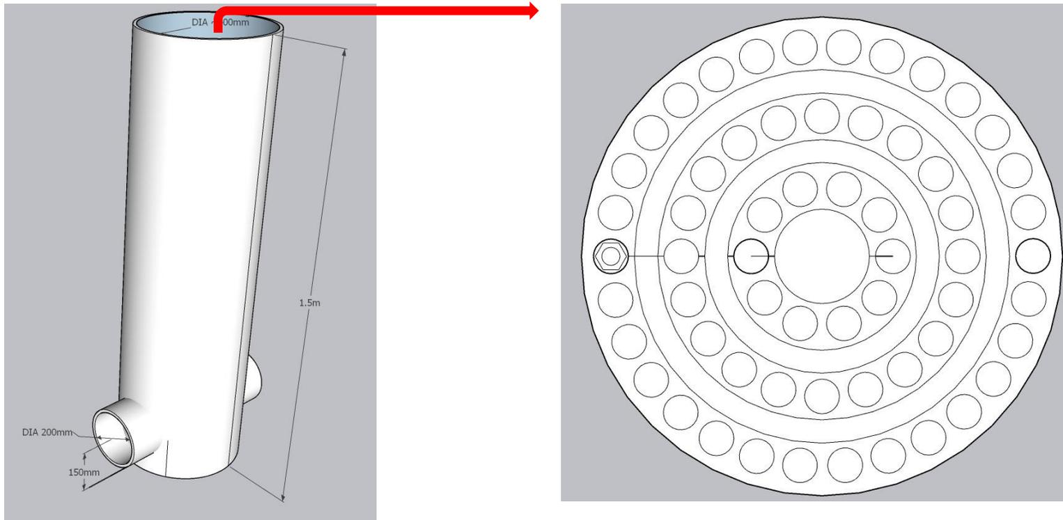
60 finned tubes are arranged in 3 rows with gaps for vapor diffusion
